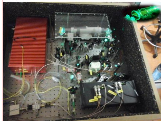
Saturated absorption technique Multi-pass sealed iodine quartz cells (length ~ 20 cm)
